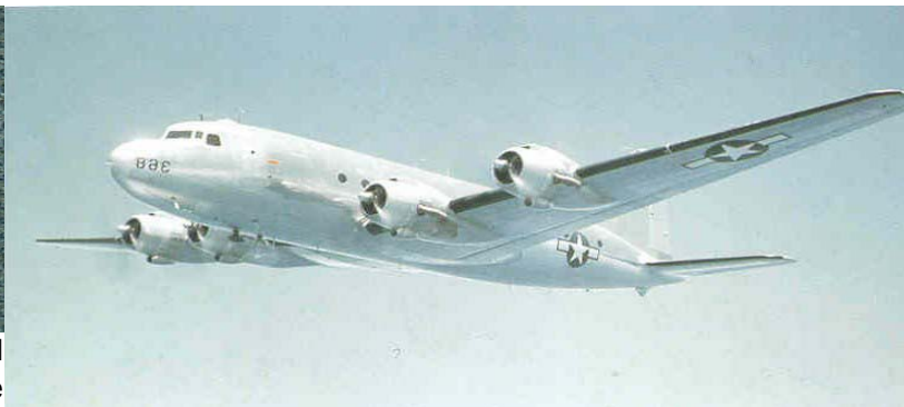
The Douglas R5D, the Naval version of the DC-4 utilizes the Pratt & Whitney R2800 Double Wasp series engines
